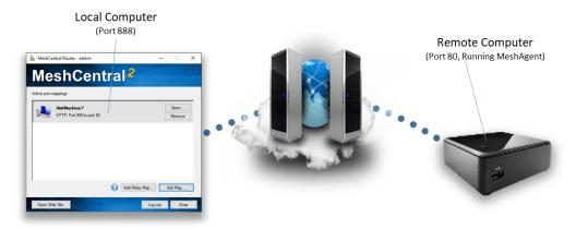
A relay port map will route traffic thru the server and thru the remote agent to a target IP address on the remote agent's network as shown here.
