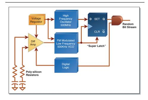
Figure 15.1 True Random Number Generator (TRNG) Hardware in Intel® AMT
