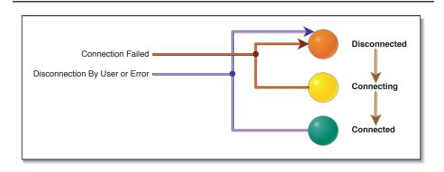
Figure 18.4 Connection State of the Manageability DTK Stack
