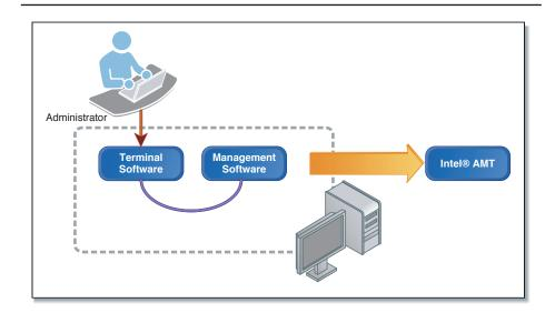
Figure 18.1 Management Software Traffic Flow When Using Separate Terminal Software
