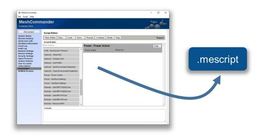
In addition to building your own scripts, you can download a CIRA setup script from a MeshCentral server. When running this script, Intel AMT will be setup to call back to the server using an encrypted connection. This enables remote management of Intel AMT over the Internet. The CIRA setup script is available in the "Add CIRA" link for meshes that are Intel AMT only (no agent).
