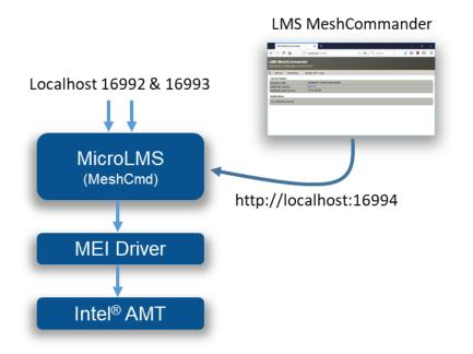
In addition to providing normal services, MicroLMS that is part of MeshCmd will also start a web server on port 16994 and allow a browser to access LMS MeshCommander, a special version of MeshCommander specially made to run in this situation.
