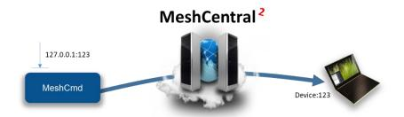
Of course, this picture is a bit simplify. Firewalls, NAT routers and HTTP proxies may be in the way and the MeshAgent on the remote computer will act at the TCP traffic relay in most cases.
